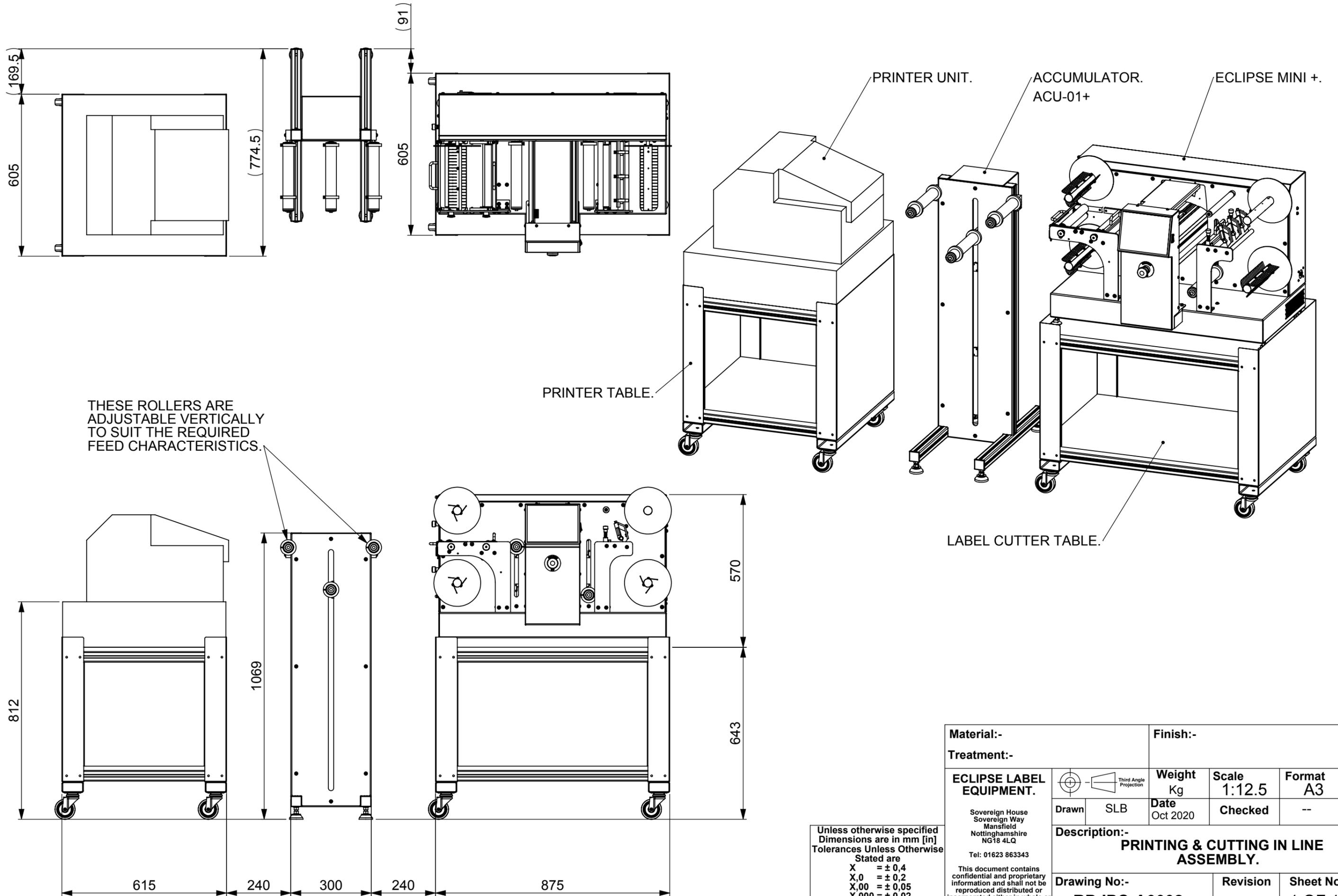
THESE ROLLERS ARE ADJUSTABLE VERTICALLY TO SUIT THE REQUIRED FEED CHARACTERISTICS.
